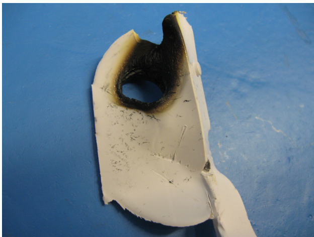
Photo after glow-wire test
